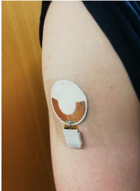
Fig.11: DDRR tag placement on the upper right arm attached via double sided tape.
