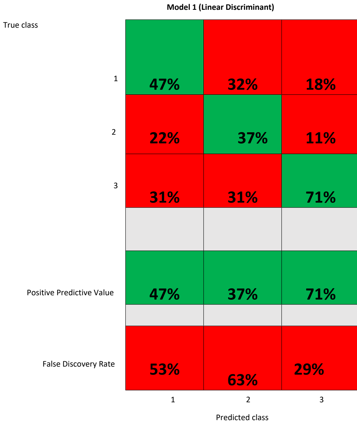
Fig. 5.54: Confusion matrix for a three-group discrimination with the aid of LDA model showing positive predictive values and False discovery rates.
