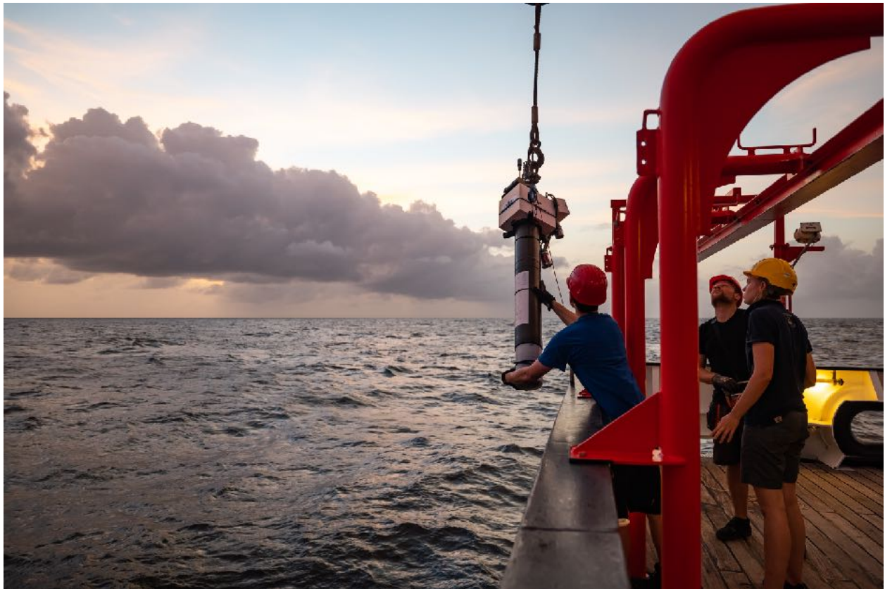
Fig. 4: Deployment of an Argo float with an Underwater-Vision-Profiler. These measurements are intended to determine the number and size of sinking particles and to obtain images of different plankton species (© David Menzel).
