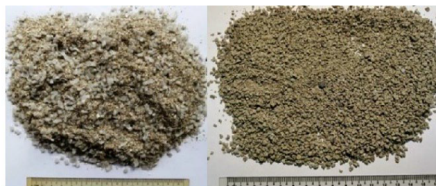
FIGURE 3. (a) kenaf composite which the polypropylene does not melt completely, (b) kenaf composite in pellet form.
