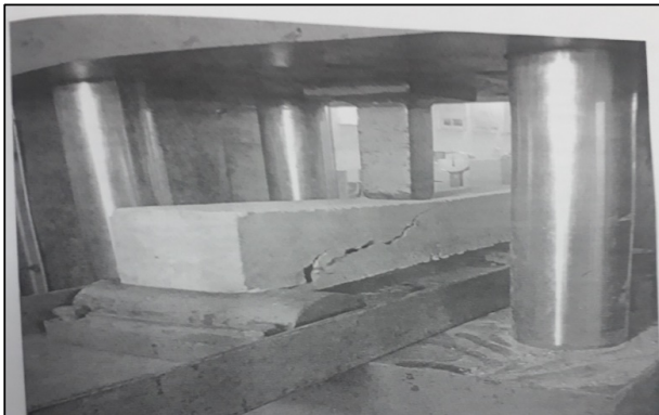
FIGURE 5. Beam subjected to Flexural Strength Test
