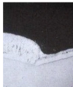
FIGURE 12. Non-Reactive and reactive steel welding together (Khode 2019)
