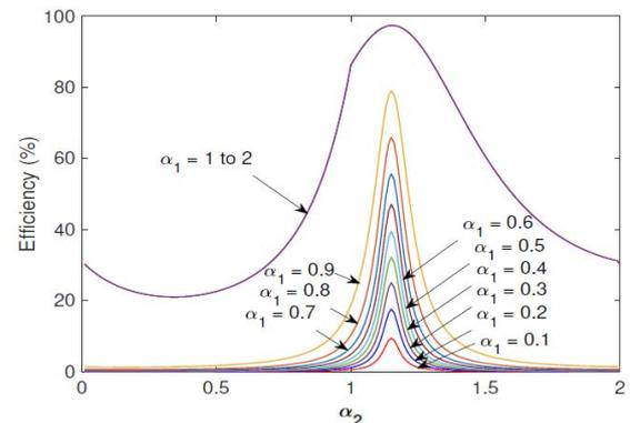
Fig. 8. Efficiency versus  $\alpha_2$  when  $0 < \alpha_1 \leq 2$  at  $\beta_{1,2} = 1$
