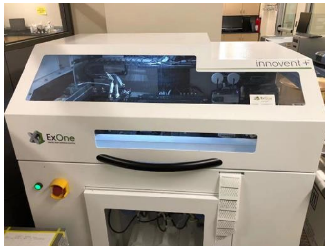
Figure 3- 3 Exone Innovent+ Direct Binder Jet Printer, University of Utah
