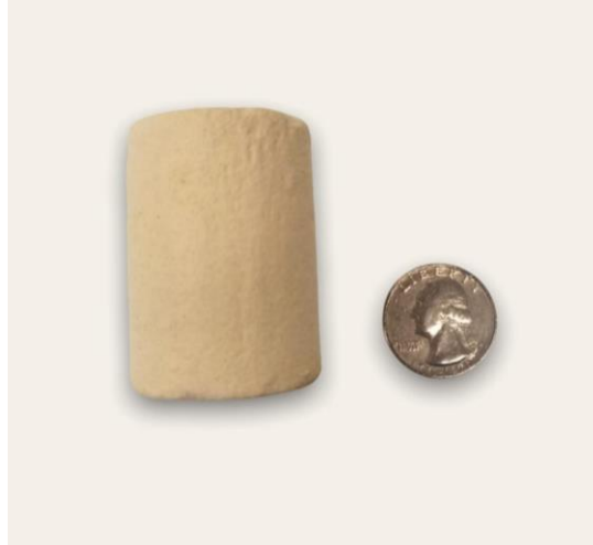
Figure 4- 4 Successful Print of Clay Powder
