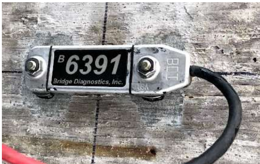
Figure 7: BDI Strain Gage
