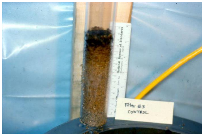
Figure 2-6. Schmutzdecke biomass development (adapted from Partinoudi et al., 2006).
