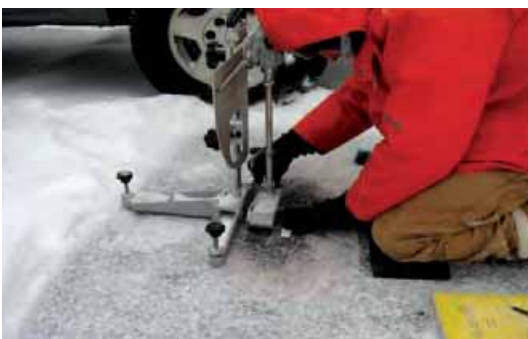
Graduate student Kris Houle measures friction resistance on a pavement during winter conditions with a British Pendulum Meter.
