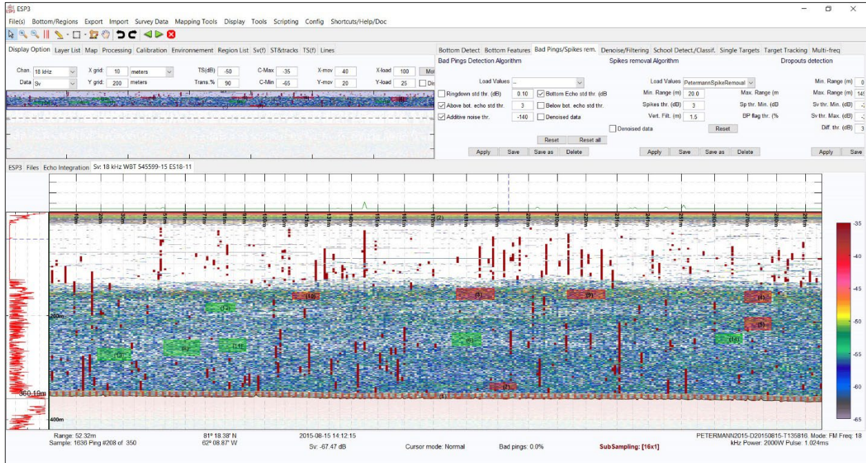
Figure 47: Higher density targets selected for S_v analysis, shown as filled red boxes; filled green boxes are lower density targets. Note that the default gain has been adjusted in this figure to bring reported signal levels closer to the calibrated signal level (see Appendix A for further discussion on the default gain and its impact on echogram images). Echogram is not calibrated.
