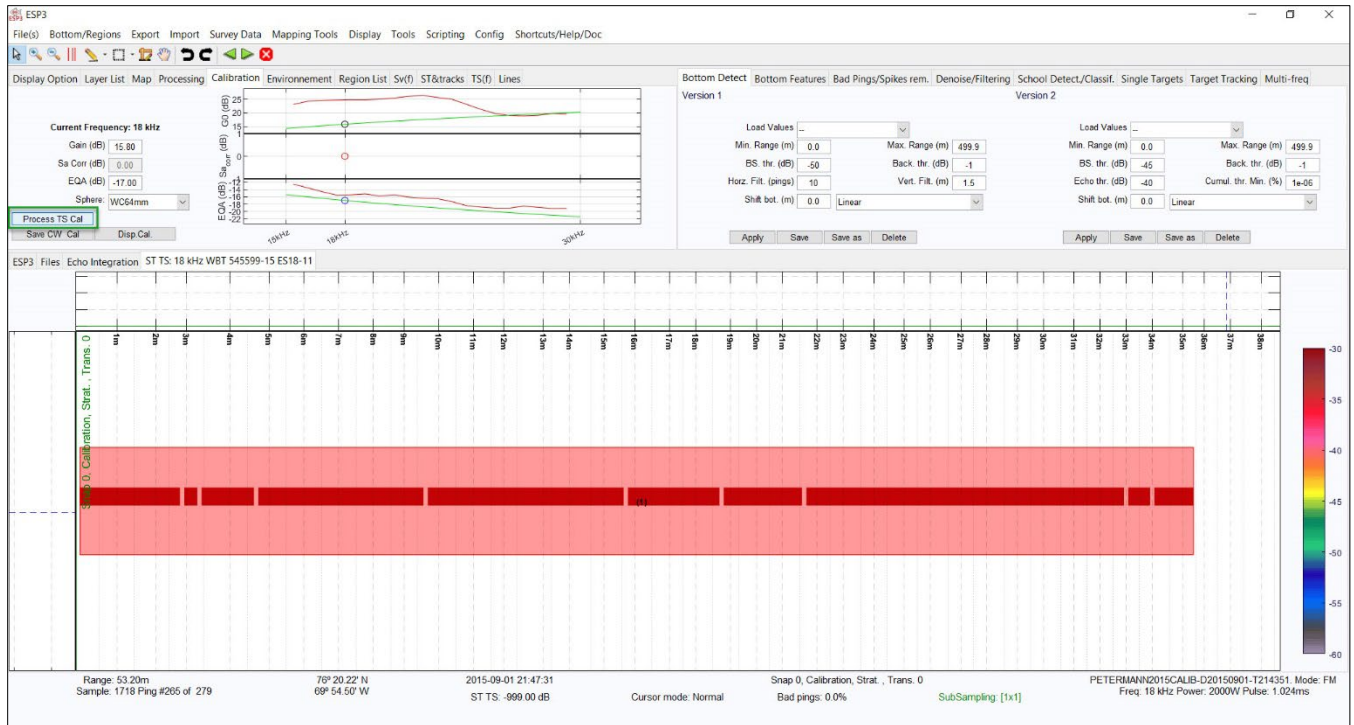
Figure 118: The calibration sphere is auto-extracted as a single target by the ESP software as the first step in the calibration processing. The green box is highlighting the Process TS Cal tool.
