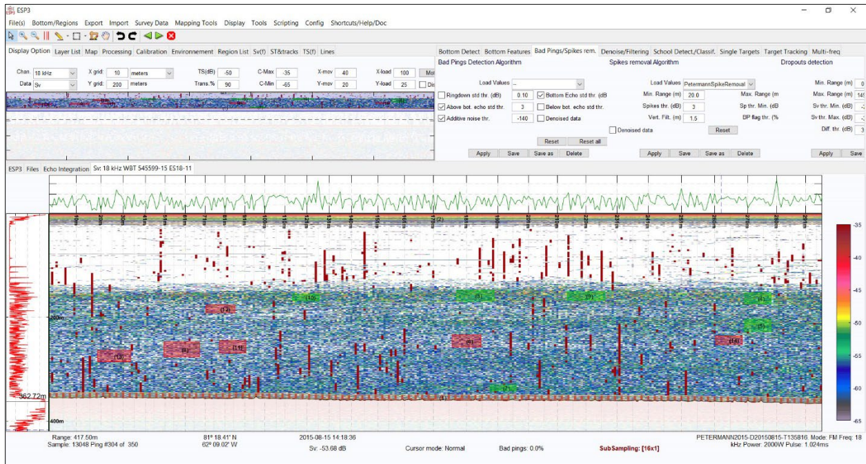
Figure 48: Lower density targets selected for S_v analysis, shown as filled red boxes; filled green boxes are higher density targets. Note that the default gain has been adjusted in this figure to bring reported signal levels closer to the calibrated signal level (see Appendix A for further discussion on the default gain and its impact on echogram images). Echogram is not calibrated.
