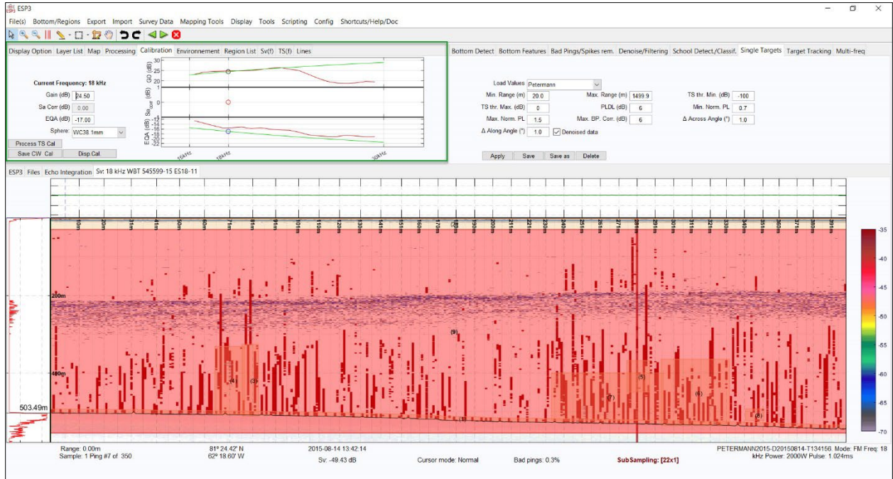
Figure 284: Echogram with "rough" calibration applied. The gain has been adjusted to be closer to the calculated calibration value at the nominal frequency.
