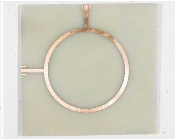
(d) Finished product after cleaning. SMA edge-launch connectors not installed.
