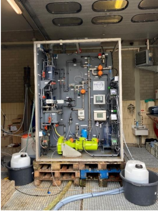
Figure 10: The front side of the CO.4 pilot that houses every component except for the ozone generator.
