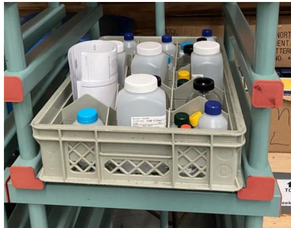
Figure 16: A set of sample bottles from HWL used for water quality analysis.
