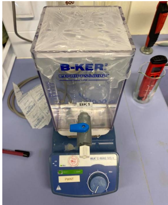
Figure 37: A fully covered jar using parafilm and filled with RWZI wastewater to the brim.
