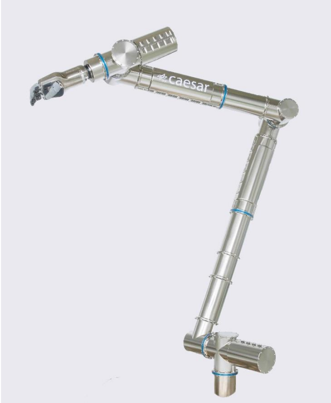
Fig. 4: CAESAR (Compliant Assistance and Exploration SpAce Robot)
