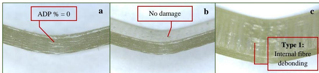
Figure 11: SP-11-GL-D50 sample photographs after programming
