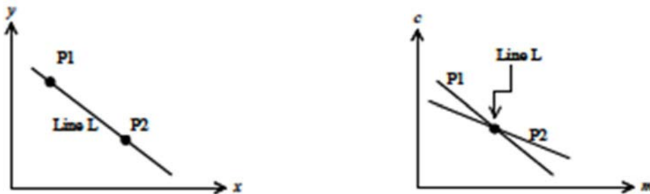
Fig. 13 and 14: The plotting of points P1, P2 on the (m, c) plane
