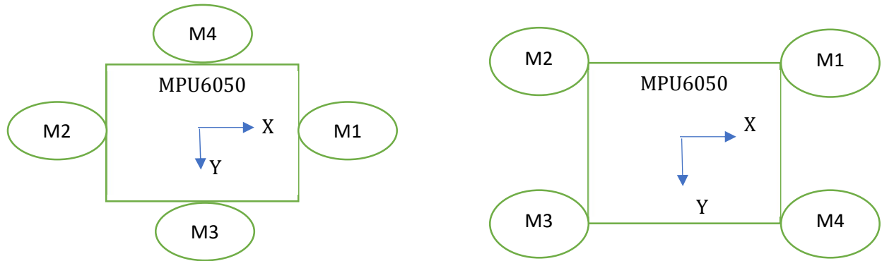
Fig. 59 Before (Left) and After (Right) Arrangement of DC Motors for SAUV Balancing
