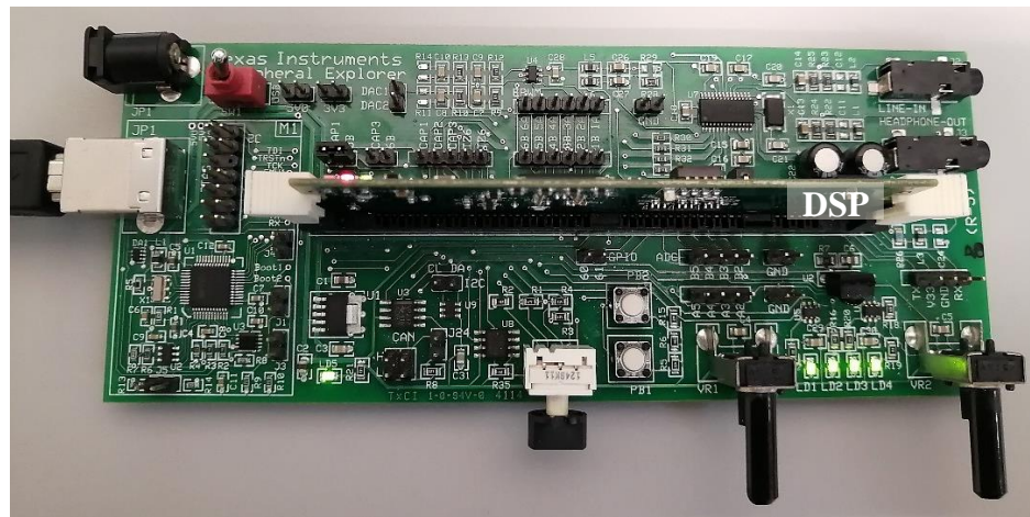
Fig. 3.4. TI docking kit with DSP for testing.
