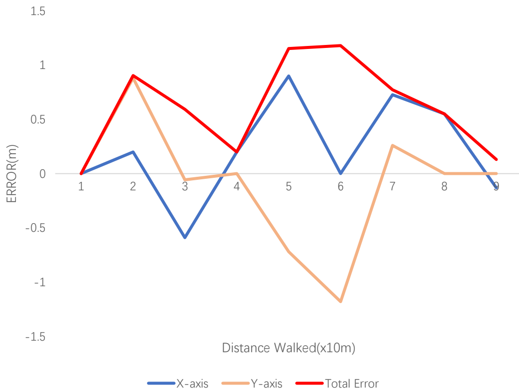
Figure 4. 8: Error line graph for the proposed ZUPT method.
