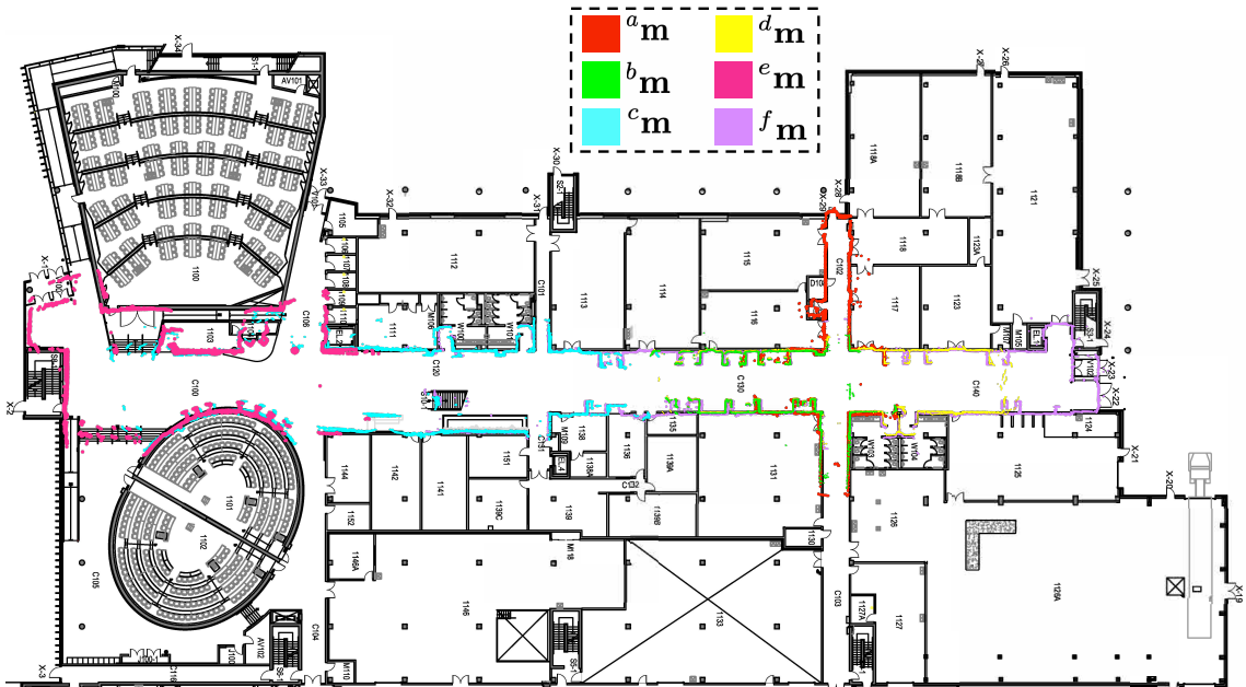
Figure 5.5: Six heterogeneous local maps obtained from different robots overlaid on the CEI building floor plan.
