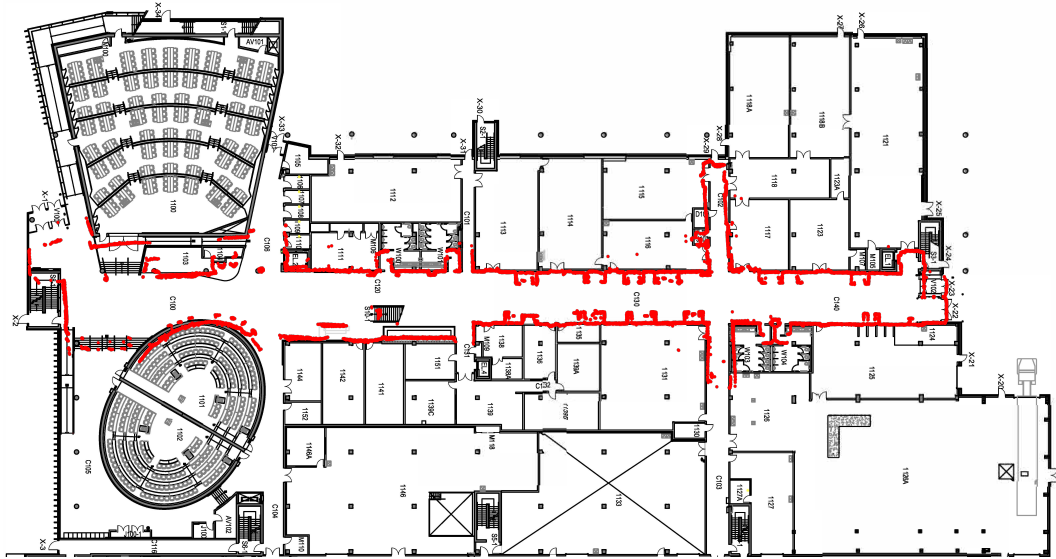
Figure 5.7: Global map obtained after hierarchical map fusion overlaid on the CEI building blueprint.
