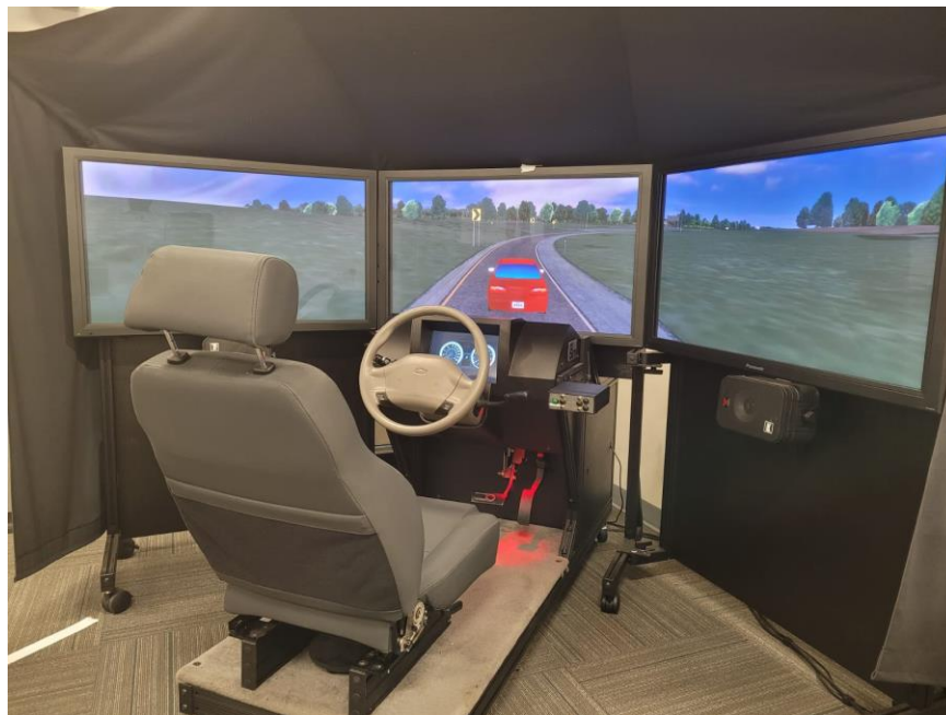
Figure 3-1. NADS MiniSim driving simulator
