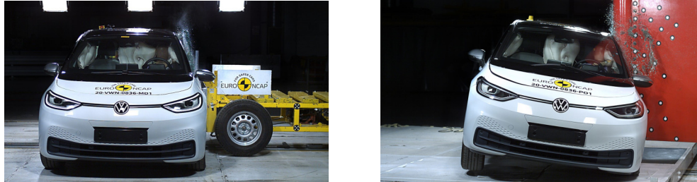
Figure 3.11: Side mobile barrier and side pole test from Euro NCAP [88]
