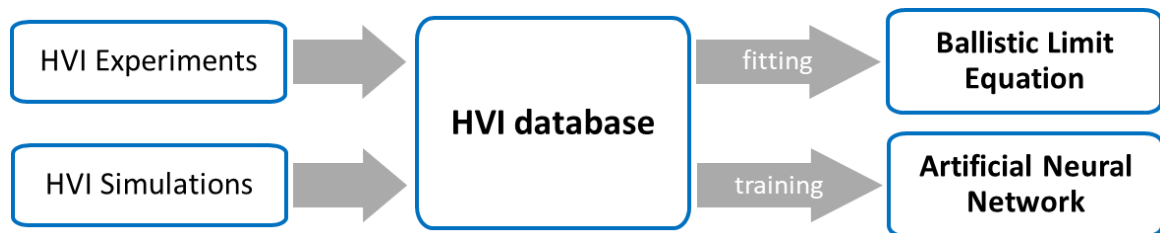
Figure 16. Development of the new predictive models (BLE and ANN) for HVI on HCSP using a hybrid database comprising experimental and modeled results.
