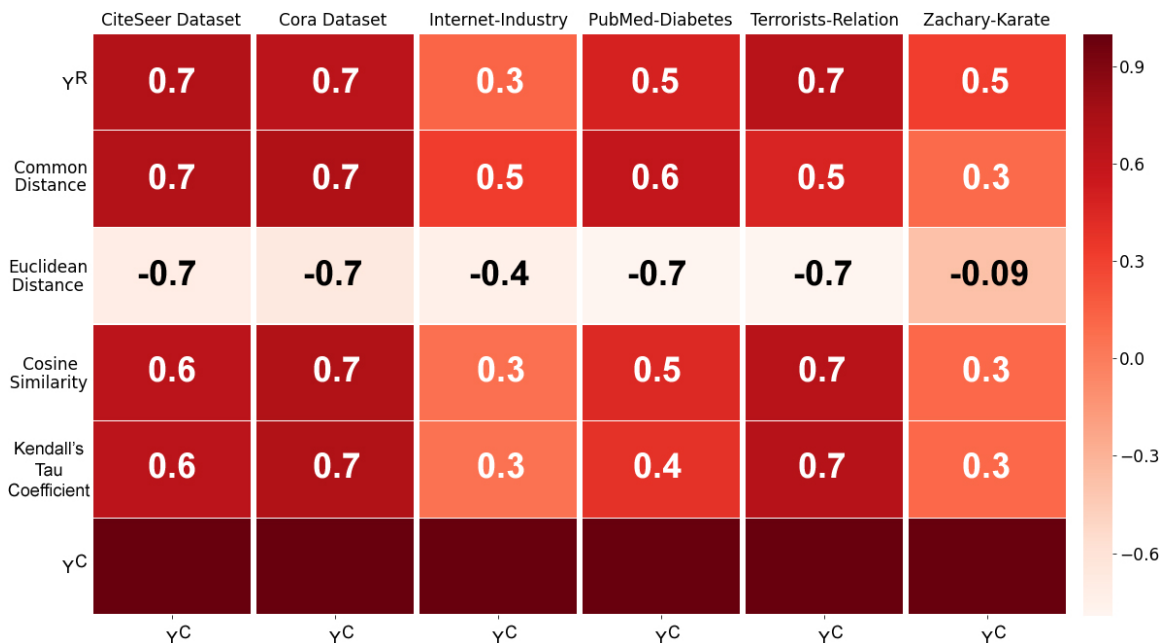
Figure 2.8: Correlation map of the prediction score or weighting proposed herein, Y^R , in comparison to other popular correlation-coefficient scoring functions.
