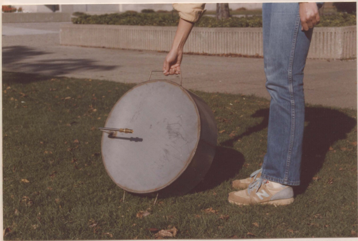
Figure 43. Seepage meter - top view.
