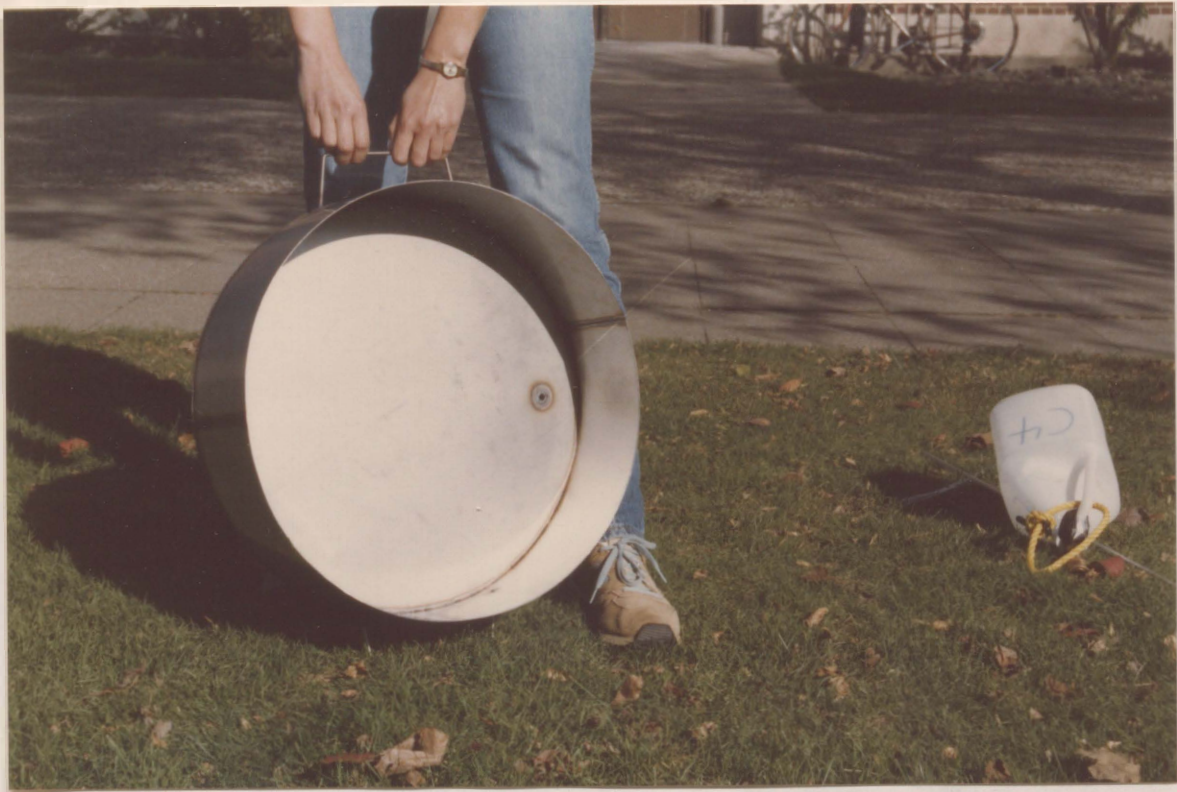
Figure 42. Seepage meter - inside view.
