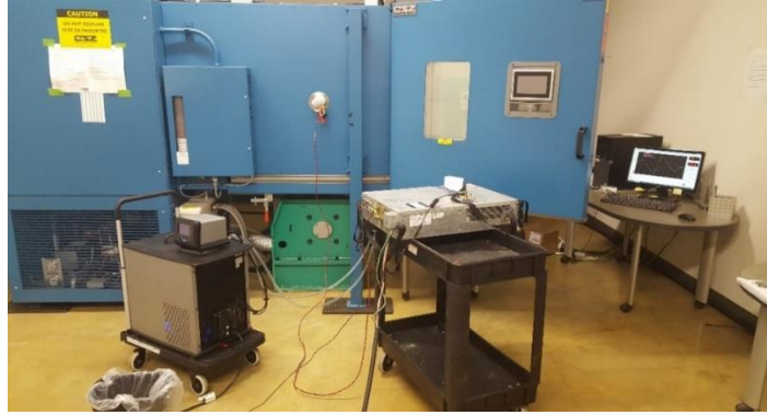
Figure 65. Vibration and Shock Chamber
