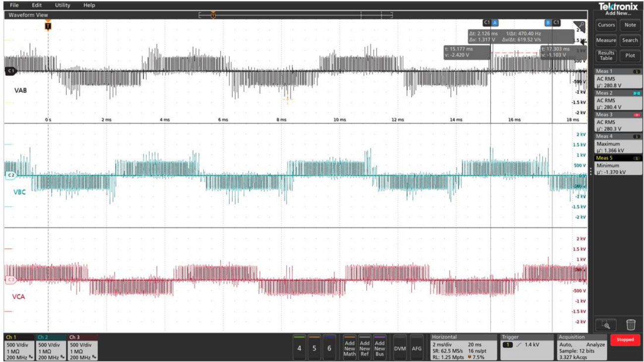
Figure 82. 650 Vdc Terminal Voltages 1020RPM Gate resistance 1.8 \Omega
