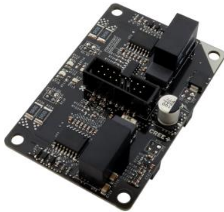
Figure 53. Wolfspeed CGD12HBXMP Gate Driver Module
