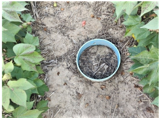
Fig. 1. Chamber collars installation and location in the study field.
