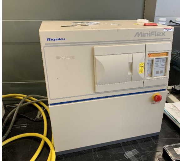
Figure D.3. A picture of Rigaku Miniflex X-ray diffractometer located in the optoelectronic lab, “Photo by Amir Shariffar”
