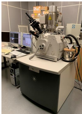
Figure D.4. A picture of the FEI Nova Nanolab 200 located in the optoelectronic lab, “Photo by Amir Shariffar”
