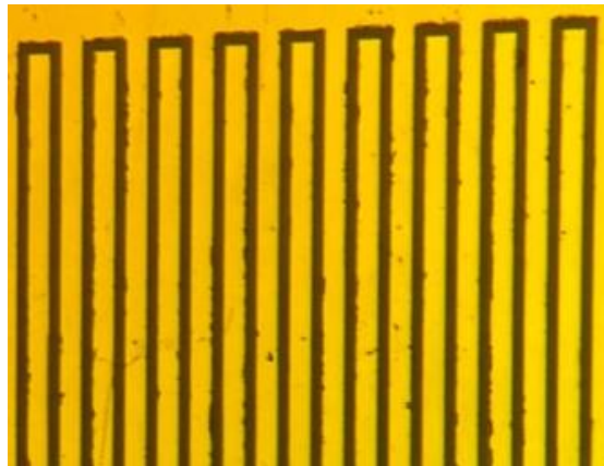
Figure D.5. A microscopic picture of the fabricated interdigital device (finger-spacing: 50 \mu\text{m} ), “Photo by Amir Shariffar”
