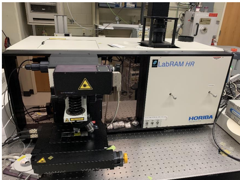
Figure D.2. A picture of Horiba LabRAM spectrometer located in the optoelectronic lab, “Photo by Amir Shariffar”
