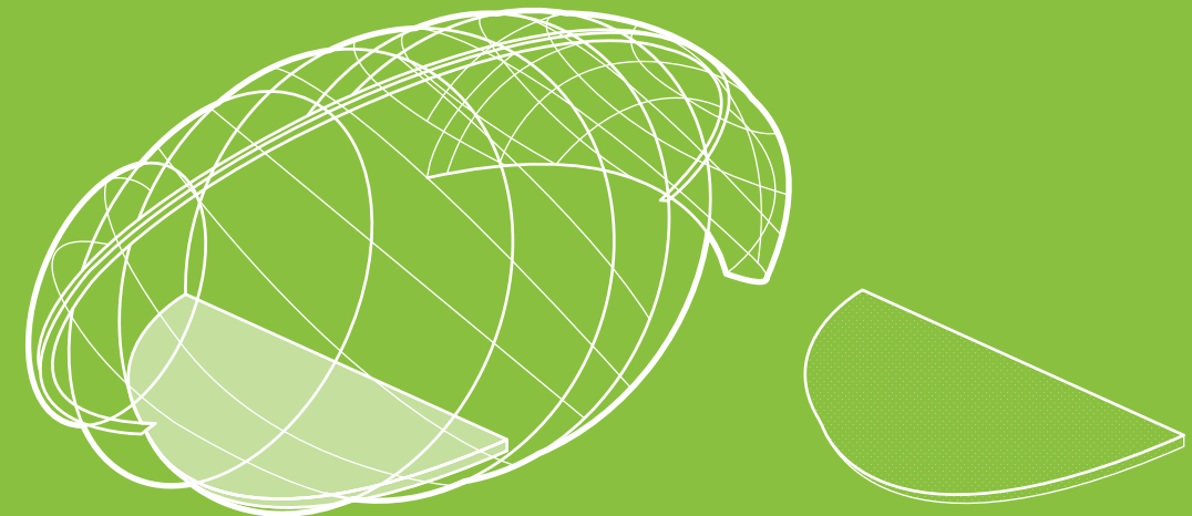
Assemble the structural frame and wooden base filled with sand
