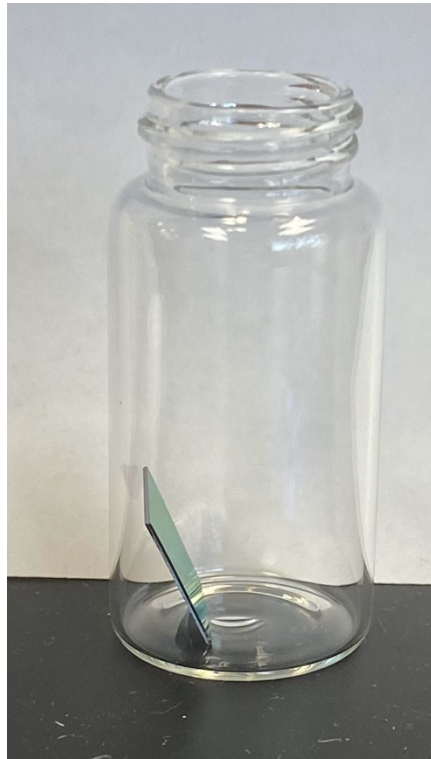
Figure 4.3 Glass scintillation vial with a piece of Si wafer angled to show the necessary step up needed for slow evaporation. During actual deposition plastic vials are used instead.
