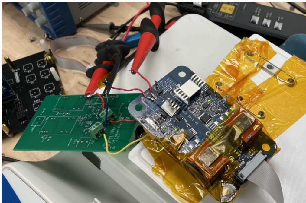
Figure 31: TSEP Board and Gate Driver Connection
