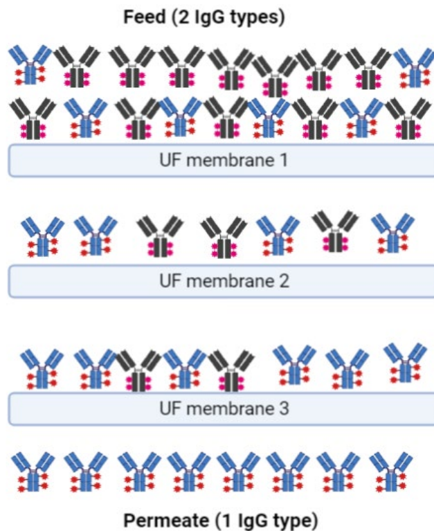
Figure 5.1: Layout of an Internally Staged Ultrafiltration System.
