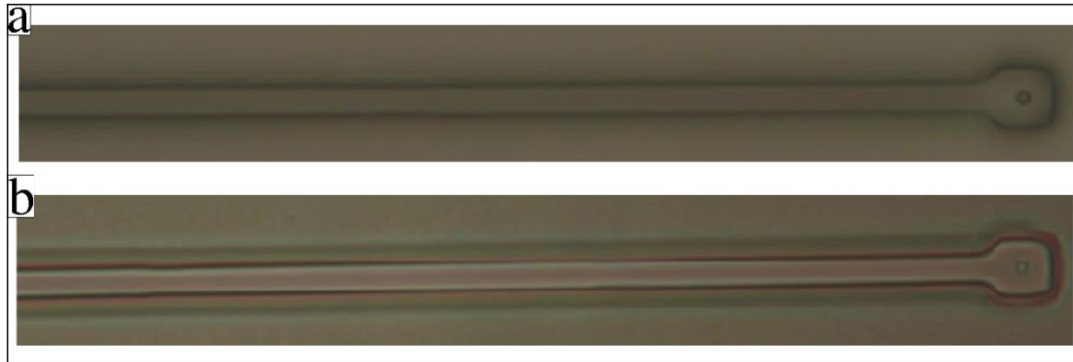
Figure 4.5: Optical images to confirm etching: (a) Optical image before HF etching, and (b) Optical images after 5 minutes HF etching and resist removal.
