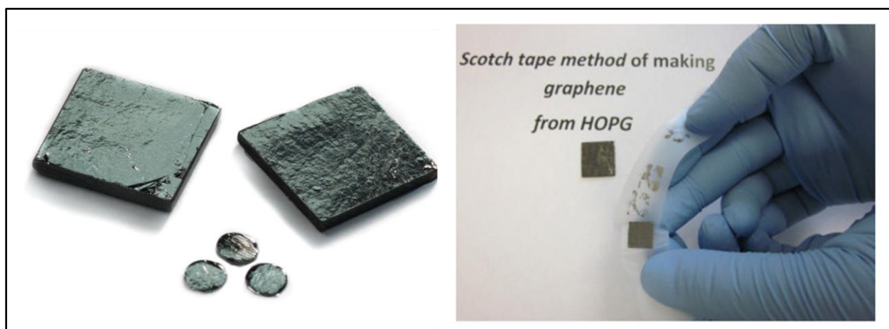
Figure 1.4: Graphene scotch tape exfoliation method from a HOPG crystal. Figure adapted from [83].
