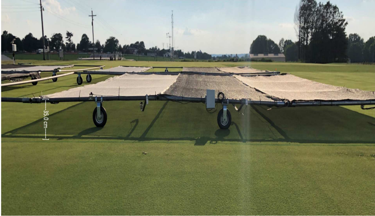
Figure 2. Transportable shade structures used to apply shade at different intensity levels.
