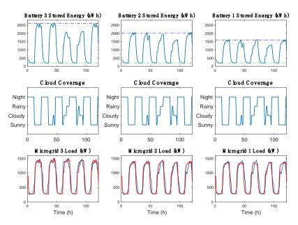
**Figure 4.** Simulation results when MGs 1–3 are *interconnected*: battery energy variation (top figure), cloud coverage (middle figure), commercial load (blue) and load power usage (red) (bottom figure).
