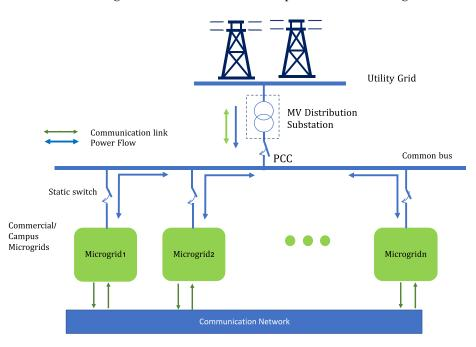
**Figure 1.** Schematic of multiple MGs that are connected to a common bus by static switches and can exchange information via a communication network.
