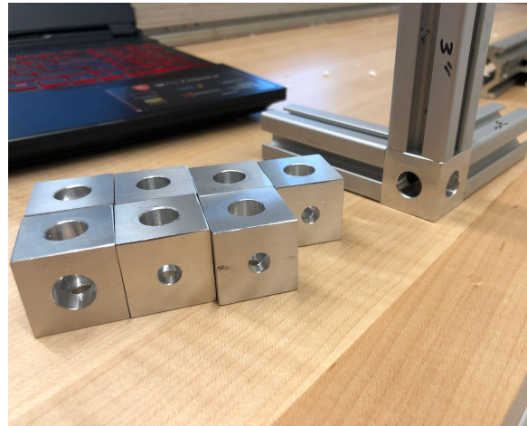
Figure 6.4: Fabricated Three-Way Outside Corner Bracket
