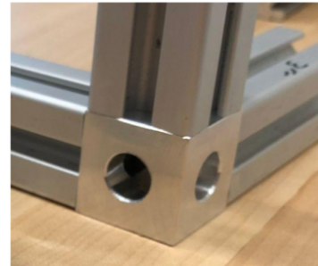
Machined corner bracket assembled with t-slotted aluminum
