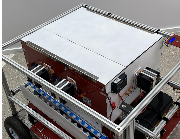
Figure 4.8: Final Refrigeration System Assembly
