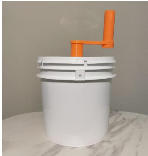
Figure J6. Bitter leaf washer fully assembled.
