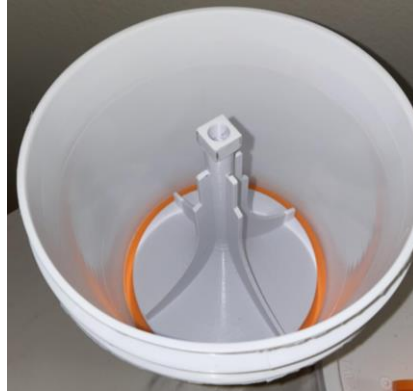
Figure O2. Agitator on top of mount inside bucket.
