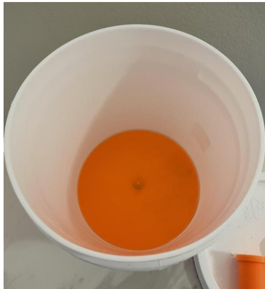
Figure J3. Bucket with agitator mount fastened to the bottom.
