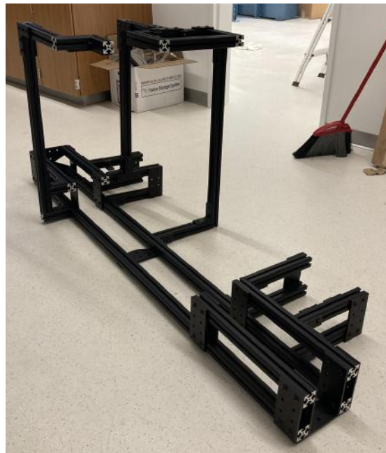
Figure 6.1: Complete Bike Rack Assembly Frame
