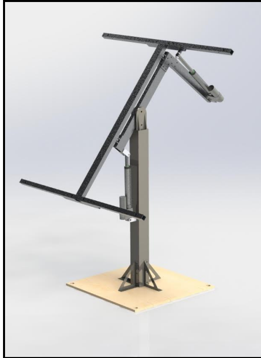
Figure 4: CAD rendering of the final actuation and structure subsystem. The actuation and structure subsystem is responsible for movement of the panel, as well as supporting the weight of the panel and system components in addition to serving as a mounting point for these system components.
