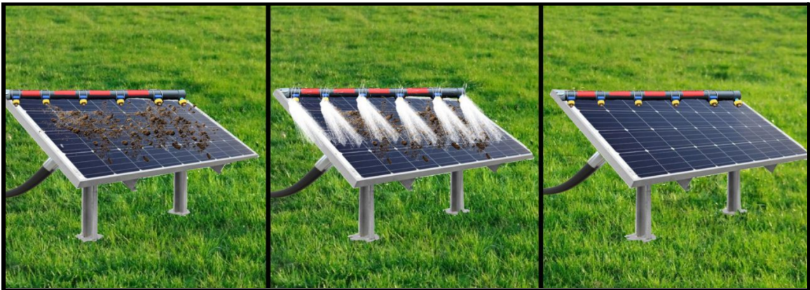
Figure 3: Concept of Operations for cleaning system. The panel is shown in a fixed position for demonstration purposes.
