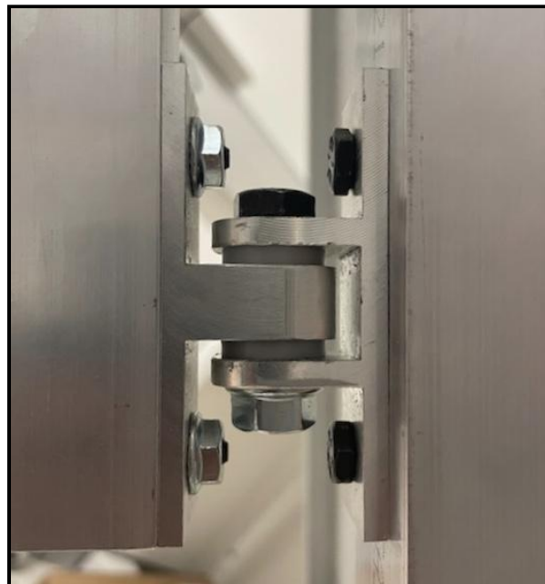
Figure 5: Close-up view of the E-W hinges connecting N-S frame to the solar panel mount. Hinges were manufactured in the SCU Machine shop under the supervision and guidance of Rodney Broome.
