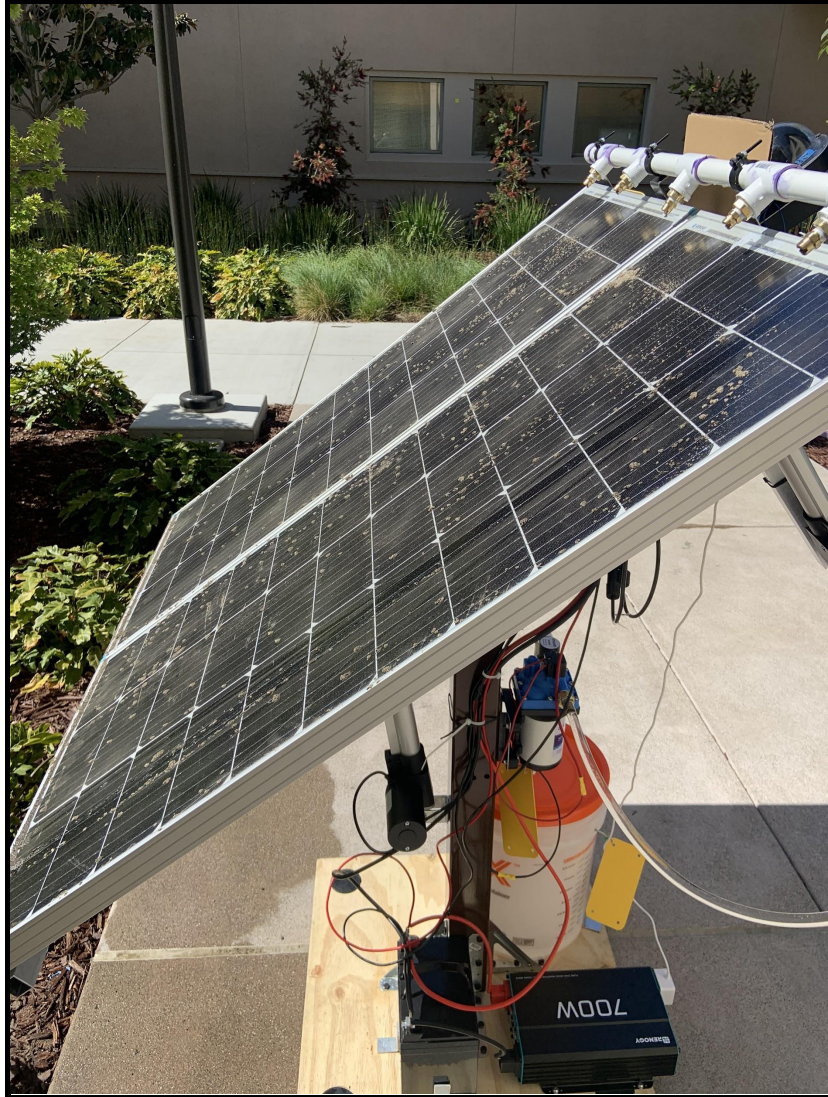
Figure 32: Depicted scenario of a dirtied panel in the worst possible conditions.
