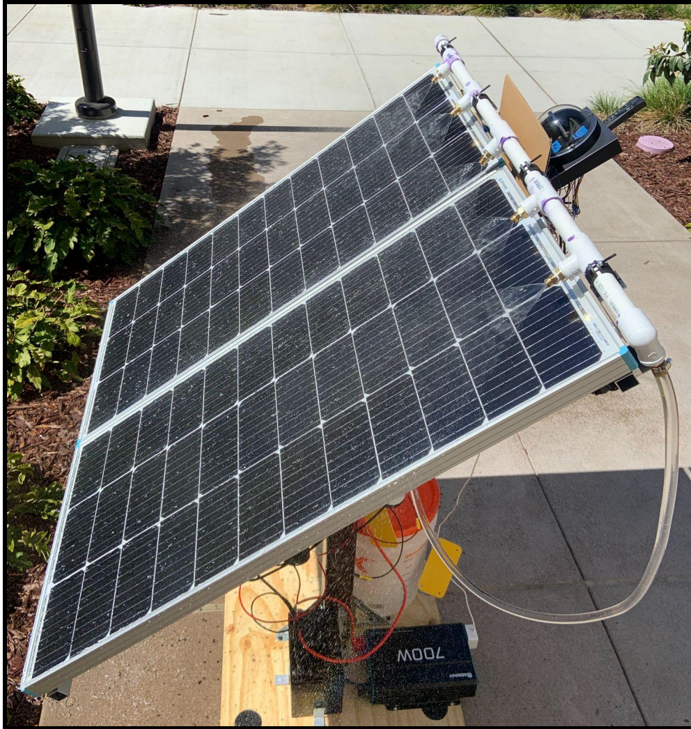
Figure 7: Cleaning system attached to the final system prototype during testing.
