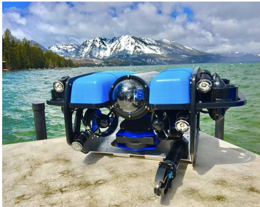
Figure 1.8: BlueROV with Newton Gripper [14].
