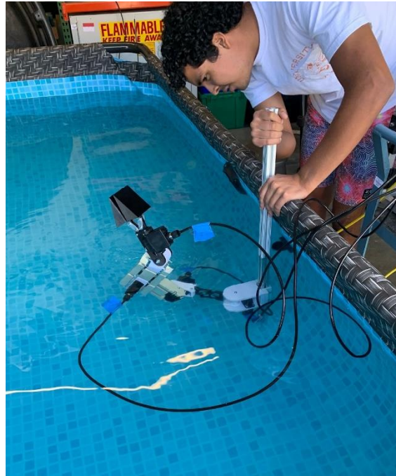
Figure 5.2: Testing manipulator in pool
