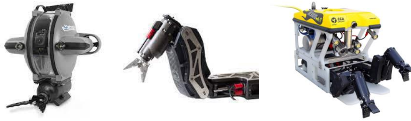
Figure 3.3: Existing Underwater Manipulator Arms from left to right: Deep Trekker Two Function Arm (Deep Trekker), TMI-Orion Electric Manipulator (TMI Orion), Arm 5e Mini [21, 19, 20].
