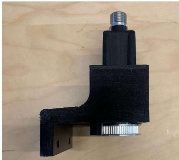
Figure 3.16: Sample storage system servo fixture to secure servo and big gear to ROV frame.
