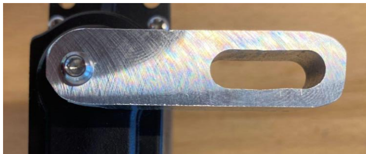
Figure 4.3: Machines slots with hand sanded rounded corners.
