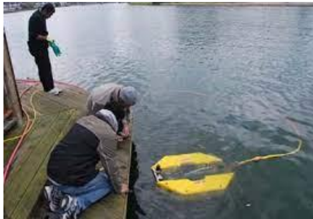
Figure 1.3: Triton RSL ROV [10].
