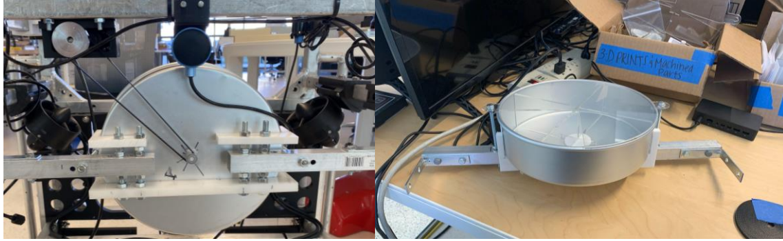
Figure 3.18: Sample Storage System assembled at end of the quarter (from below the robot and before installation).
