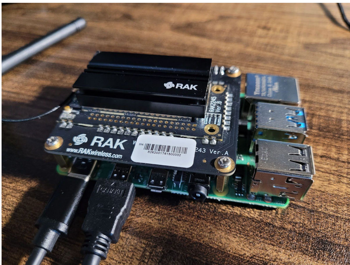
Fig. 3.2: Raspberry Pi with RAK2245 Pi Hat Mounted
