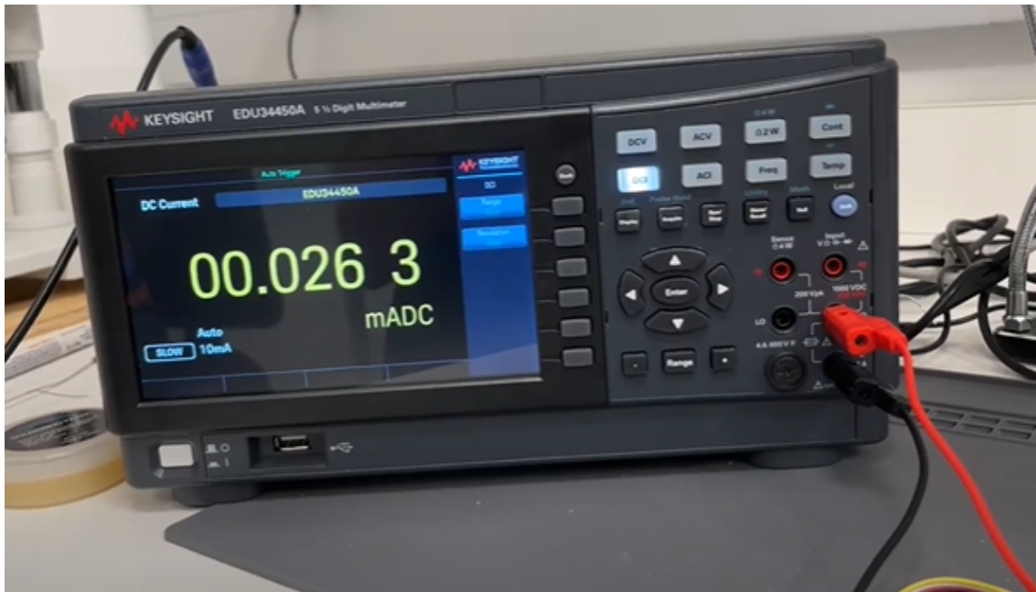
Fig. 3.8: Arduino Sleep Current Measured on Digital Multimeter
