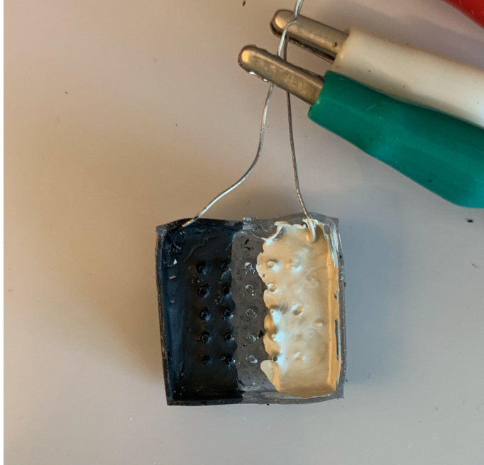
Figure 3-9: Final microneedle array after electrode fabrication
