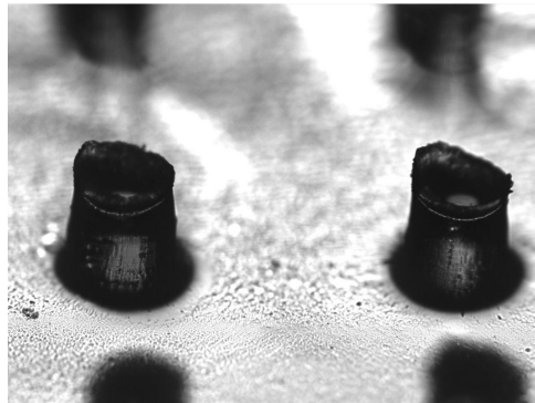
Figure 3-7: Unsuccessful microneedle pattern transfer to PDMS mold
