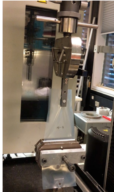
Figure 3. Tensile testing in a sample fixture perforated with a mandrel arranged for the purpose.
