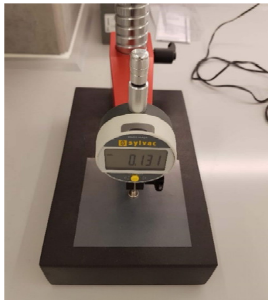
Figure 5. Mechanical thickness measurements of a sample using a dial gauge from Sylvac.
