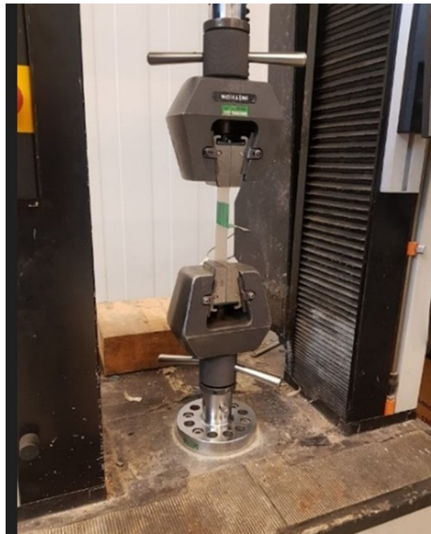
Figure 9. Instron test machine for measuring the adhesive strength.
