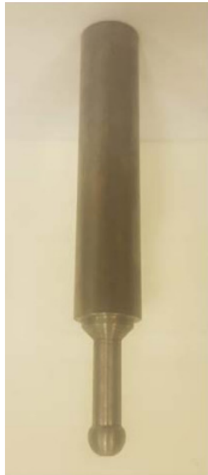
Figure 4. Drop weight and ball weighs 500 \text{ g} \pm 5 \text{ g} and has a diameter of 12.7 \text{ mm} .
