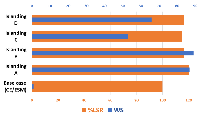
FIGURE 6. Comparison of DCOPF formulation based base case (CE/ESM) and DCOPF formulation based IIS for IEEE 118-bus system.
