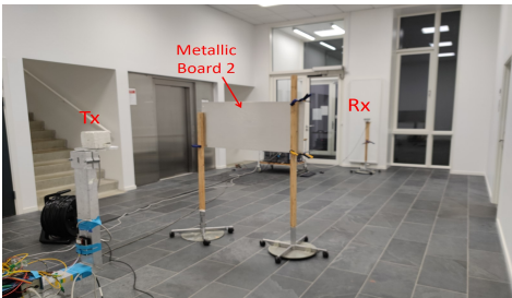
Fig. 1. The illustration of the measurement room (a) and measurement photographs taken in (b) the LoS scenario, (c) the OLoS1 scenario, and (d) the OLoS2 scenario.
