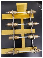
11) Set the assembly into the main bioreactor box, attach designated polypropylene tubes to their cannulas, and if necessary secure brackets to the bioreactor box and remove static rods. Sterilize by running 70% ETOH through the scaffolds in seeding mode for 30 min. Rinse 3 times with PBS and wet with cell media 24 hrs prior to seeding.
