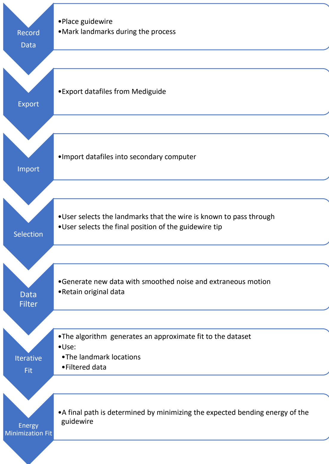
Figure 54. Diagram of the algorithm procedure to determine the optimal guidewire path.
