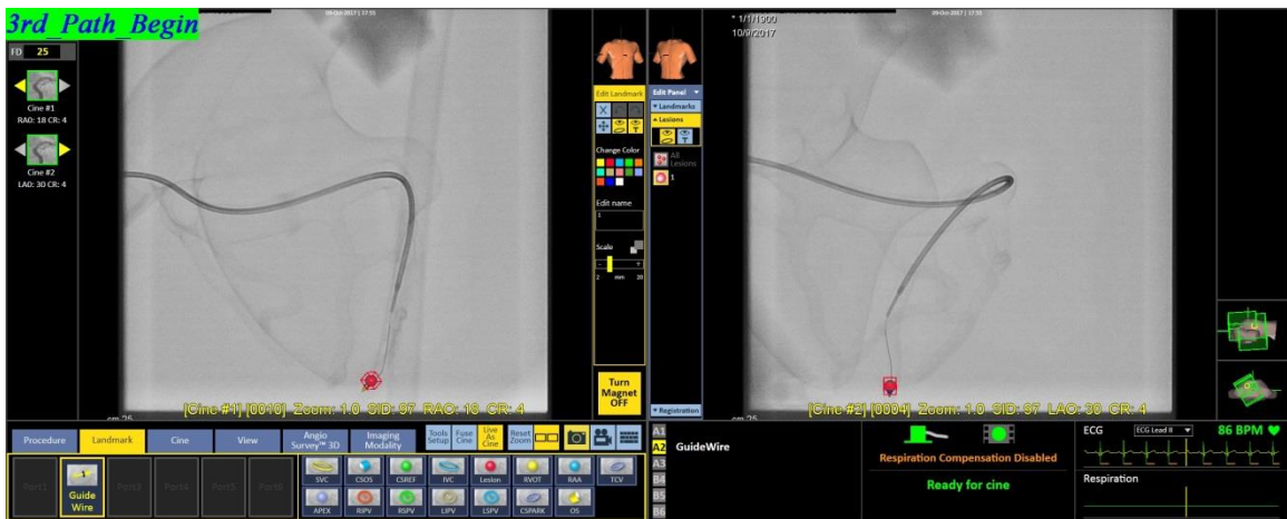
Figure 55. Biplane MediGuide display of the placement of a landmark in the distal portion of an artery in a coronary phantom.
