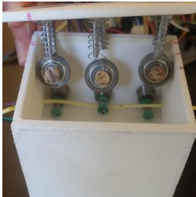
Figure 23. The rotary encoder measurement device with the lid utilizing spring loaded bearings to maintain pressure on the catheter. [30]
