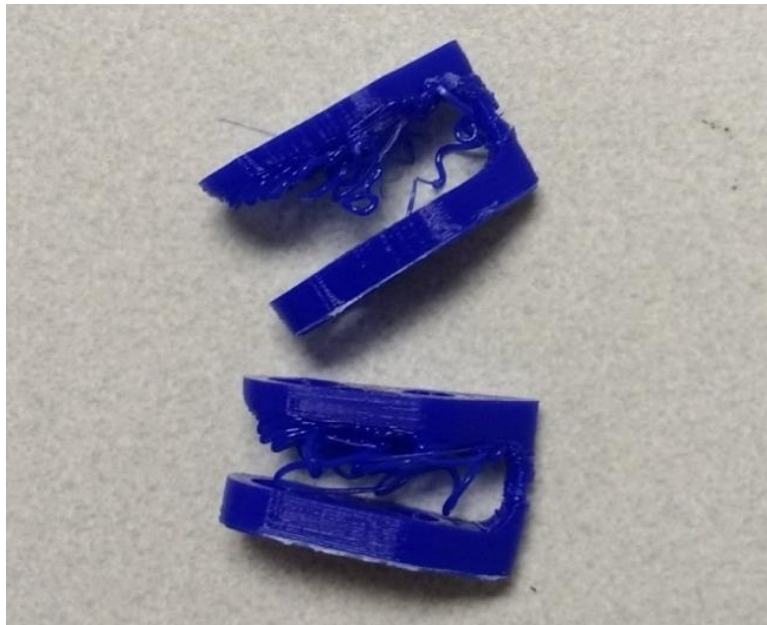
Figure 34. Second iteration rocker link that proved difficult to 3D print and needs to be redesigned to function properly.
