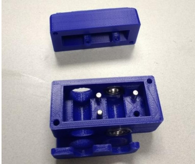
Figure 33. Second rotary encoder prototype device iteration partially assembled.
