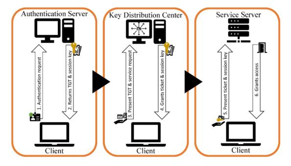
Figure 1. Kerberos authentication process
