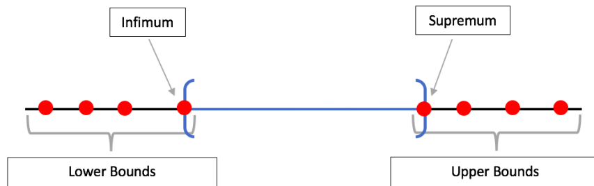
Figure 23: Graphical representation of supremum, infimum, upper bounds, and lower bounds on the open interval (a, b) .
