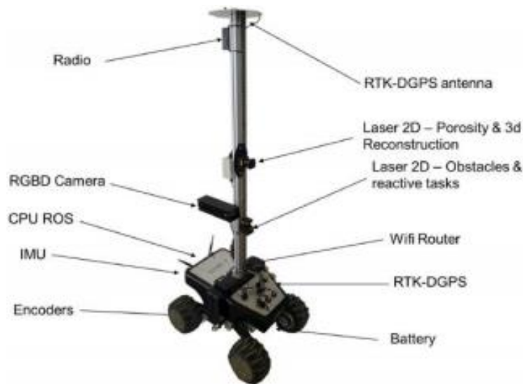
Figure 10. Vinbot component sensor and component distribution (Guzman et al., 2016)
