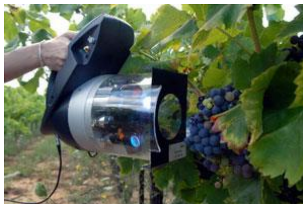
Figure 1. Multiplex hand-device sensors for quality of grape (Matese and Di Gennaro, 2015)
